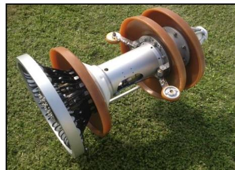
The data-recorder contains all power, processing and recording circuits in a sealed module within the central body of the Caliper-Tool.
